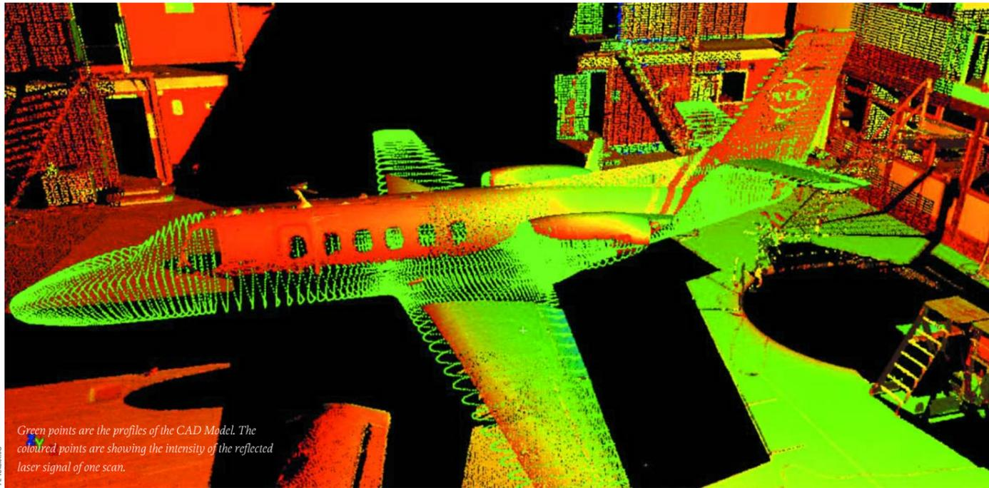
Green points are the profiles of the CAD Model. The coloured points are showing the intensity of the reflected laser signal of one scan.
