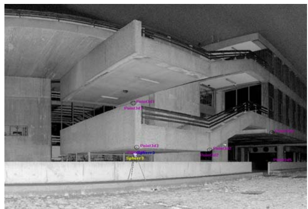
Figure 9. Registration using spherical targets in FARO Scene
