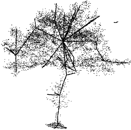
Figure 4: Example of a skeleton extracted from ALS data. The example cloud was scanned with a FLI-MAP 400 system and approximately 50 points per square meter.
