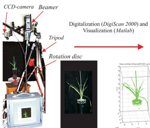
Fig.3: DigiScan2000 system, barley (*Hordeum vulgare* L.) plant in a pot and the visualization
